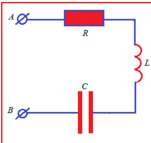
$$\begin{aligned} U &= U_R + U_L + U_C \\ U_R &= R \cdot I \\ I &= \frac{dq}{dt} = C \cdot \frac{dU_C}{dt} \Rightarrow U_C = \frac{1}{C} \int_0^t I(\xi) \cdot d\xi + U_C(0) \\ U_L &= L \cdot \frac{dI}{dt} \\ U &= R \cdot I + L \cdot \frac{dI}{dt} + \frac{1}{C} \int_0^t I(\xi) \cdot d\xi + U_C(0) \end{aligned}$$
